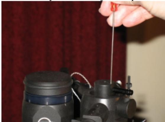
Fig.10 Fixing vertical damping holder
