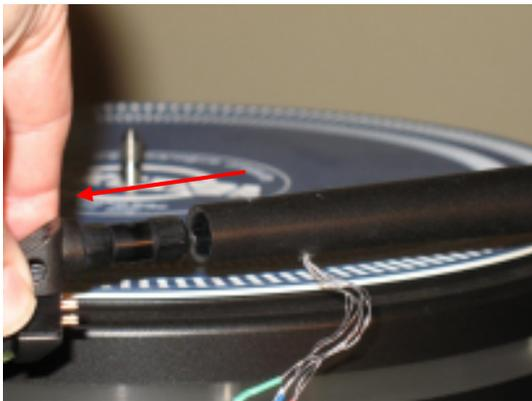
Fig.7 Removing headshell
