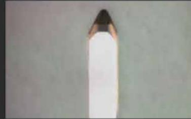
Aluminum Cantilever with Elliptical needle
