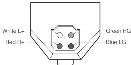
3. Fasten the cartridge to the headshell using a pair of screws enclosed the packing. Do not tighten the screws completely before the stylus unit has been remounted.
