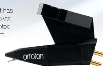
The Super OM 5 also features an improved engine with Ortofon's trademark split pole pins, an invention, which enables Moving Magnet cartridges to have a flat frequency response as with a Moving Coil cartridge.
