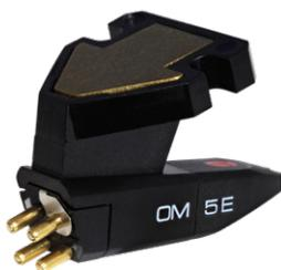
Ingeniously tucked into the top of the mounting bracket is a tiny, removable weight-plate. If your tonearm is a standard tonearm, just leave the weight-plate. If your tonearm is one of the low mass types, then simply remove the weight – the mass of your OM cartridge is now a mere 2.5 g.
