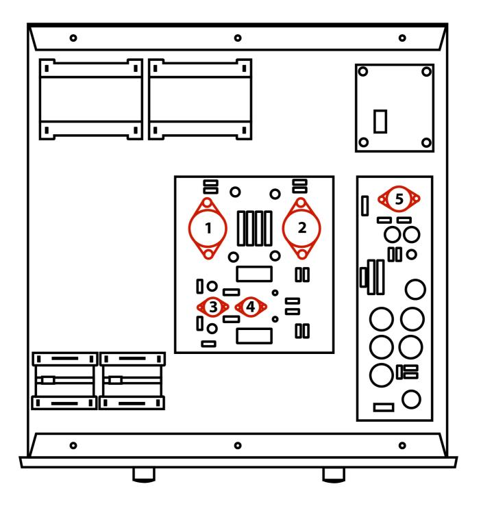
VALVE 1; 300B VALVE 2; 300B VALVE 3; 5687 VALVE 4; ECC82 VALVE 5; 5U4GB
