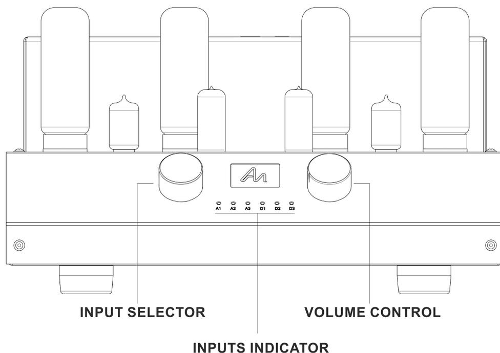
**Input Selector** Turn the input selector knob until the light of the source you wish to listen to lights up.
