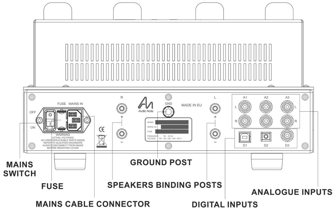
**Line inputs** Three line level inputs are available, labeled 'A1', 'A2' and 'A3', located on the right hand side of the rear panel.
