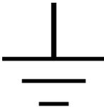
This product must be earthed – ensure that the mains supply cable earth / ground is correctly connected.
