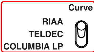
This 3 positions switch allows you to select the desired de-emphasis curve.
